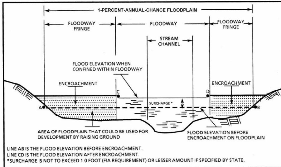
**Figure 3: Floodway Schematic**
